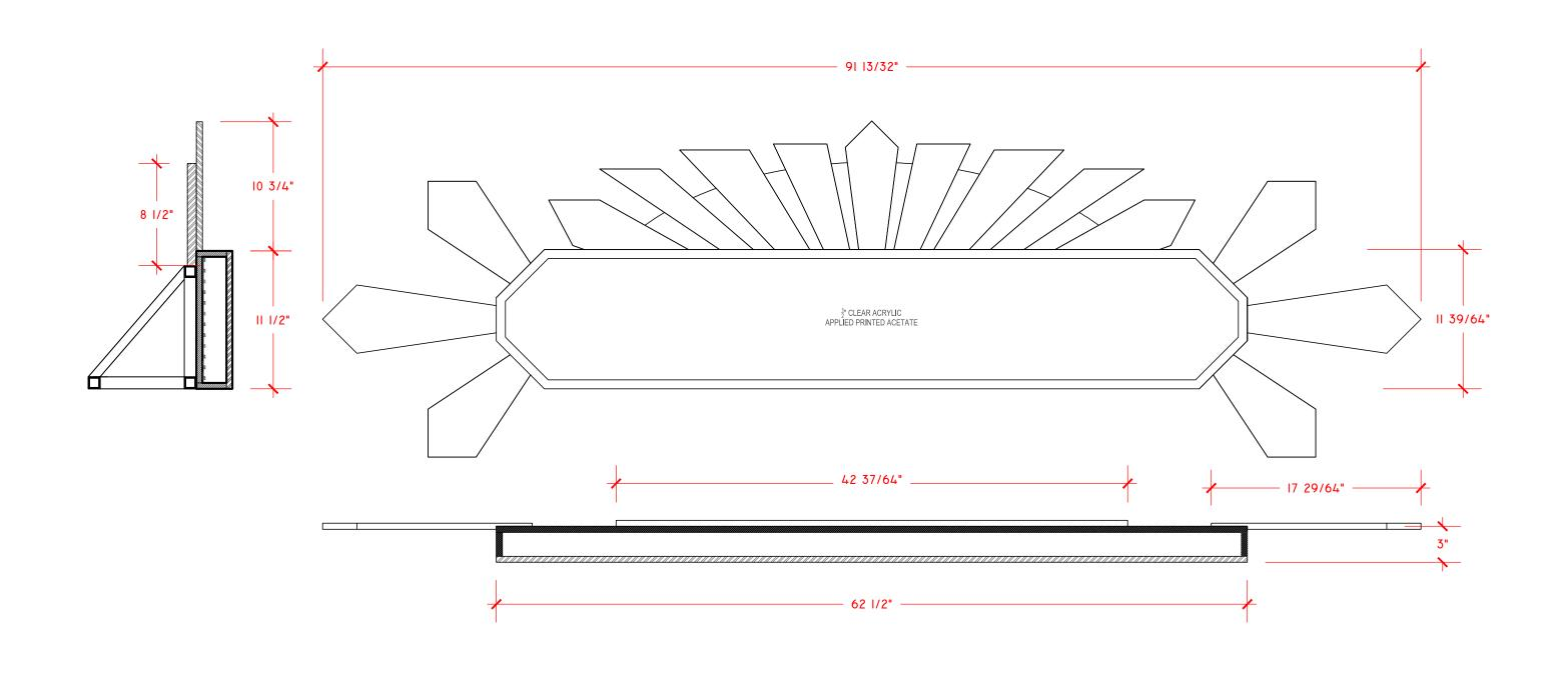
KISSING BOOTH HEADER - PLAN AND ELEVS SCALE: 1-1/2"= 1'-0"
